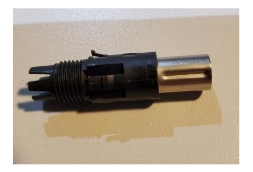
If you do not seat the pin assembly correctly in the plastic housing, these pieces will not fit correctly in the outer housing.
