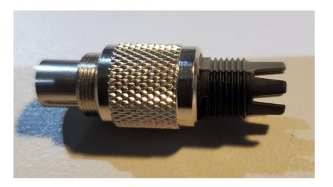
Slide the pin assembly + inner housing + plastic housing all the way into the outer housing.
