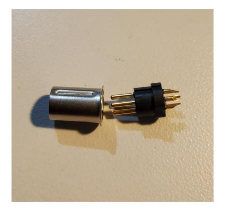
The pin assembly slides into the metal housing. Note that the housing is grooved such that the pin assembly can only fit in in one orientation. Also note that one end of the metal housing is beveled – so note the orientation relative to the pin assembly.
