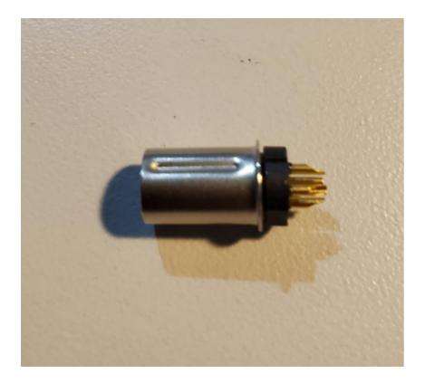
The pin assembly should sit flush against the beveled end of the metal housing.
