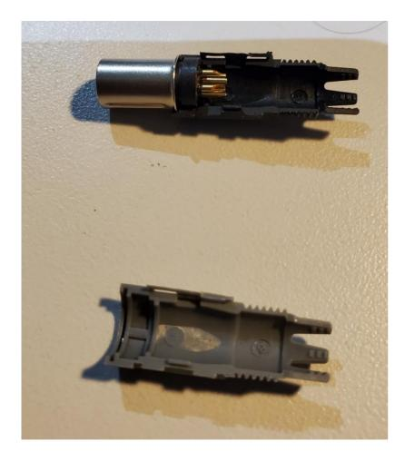
The two halves of the plastic housing go on next. Note that the plastic housing pieces have a thin groove which mates with the beveled end of the metal housing.
