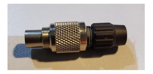
Finally, screw the last plastic piece onto the threaded end of plastic housing to crimp down on the cables.
