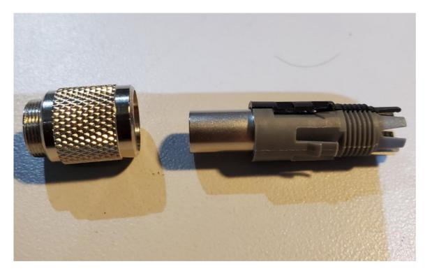
The end of the inner metal housing goes into the outer metal housing in this orientation.
