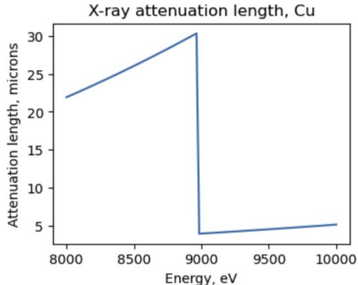
To be homogenous enough means particles shall be **smaller** than the attenuation length
