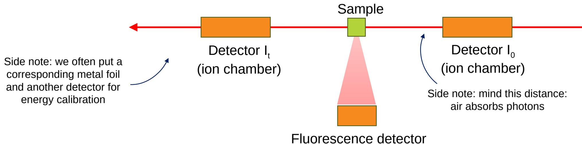
Fluorescence: emitted photons are collected by the detector placed on the side of the sample
